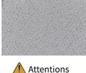
color change; incomplete or damage of shape; Dead color, without translucency. b.Check whether there is adhesion. If yes, separate zirconium beads to ensure the good liquidity. c.Qty:Completely cover the sagger bottom, 2-3 layers. d.When changing new beads, have the beads with waste sintered for 1-2 times,
