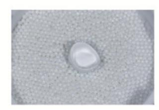
Put the restorations occlusal surface down on the zirconium bead; Follow the sintering curve as below.
